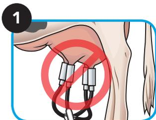
**DO NOT** remove LOCKOUT by action of milking machine.
